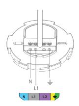
Install the wires as shown.
