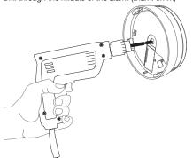
Install the power supply unit into the mounting base ring or use the conduit box as shown in option 1 & 2.
