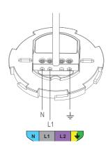
Screw the mounting base on the ceiling.
