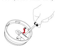
Replace the battery respecting the polarities. Attach the alarm on power supply unit by twisting clockwise until it clicks, and test the alarm.
