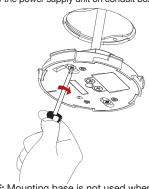
**NOTE:** Mounting base is not used when the alarm is installed on conduit box.
