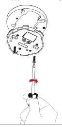
Once the mounting base with power supply unit is installed, attach the alarm by twisting clockwise until it clicks. If the battery is either missing or inserted incorrectly, the smoke alarm will not be able to click into the mounting base.
