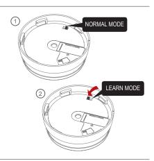
Please note: The learn switch placed on the back of the alarm can only be in learn position when the alarm is disassembled from the power supply unit. The learn switch will automatically switch to normal position when the alarm head is fitted to the power supply unit.
