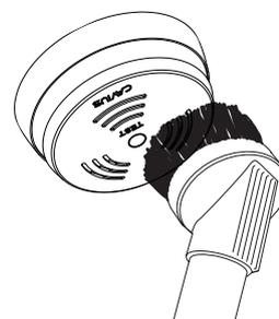
**NOTE:** You can easily vacuum clean the smoke chamber through the dedicated slot in the top cover, and it's possible to test the alarms by pressing the cover at the same time.
