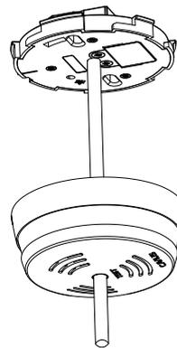
Connect the 4 wires to the power supply unit: Live feed (L1), neutral (N), Ground (≡), lamp feed wire (L2).
