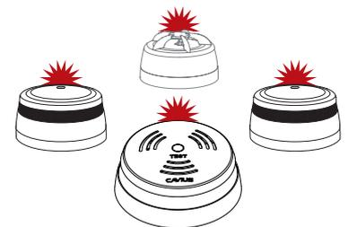
When all alarms flash the red LED, they are connected and can be switched out of 'Learn Mode' and installed.
