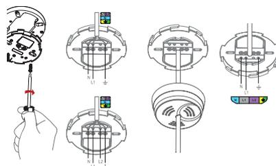
Install the cableholder and replace the cover.
