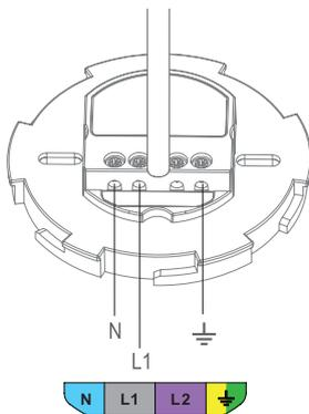
Screw the mounting base on the ceiling.
