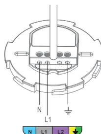
Screw the power supply unit on conduit box.
