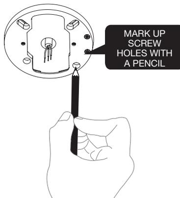
For surface wiring pass the feed wire through the mounting base cable holder and screw after termination.
