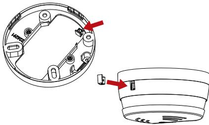
Place the Safety lock into the slot once the alarm has been clicked into the base. To remove the Safety lock in future, you will require a screwdriver and we advise to not be too forceful when removing.
