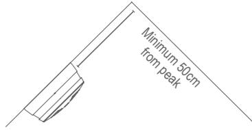
**5. INSTALLING THE SMOKE ALARM:**
