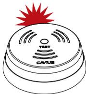
Do not remove the battery during 'Learn Mode' as this will interrupt the learn process. Press and hold the test button on one alarm only, until it beeps and the LED flashes. This alarm will become the master and will start sending out a specific house code to the other alarms.
