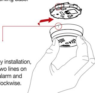
**TIP:** For easy installation, line up the two lines on the smoke alarm and PSU, turn clockwise.
