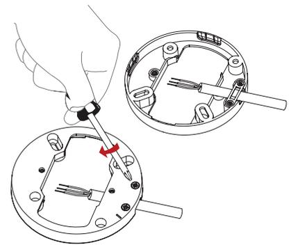
Connect the 3 wires to the power supply unit: Live feed (L1), neutral (N), Ground (⊕).
