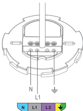
Install the wires as shown.
