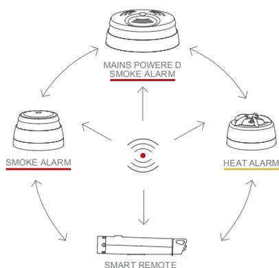
The mains powered smoke alarm can be used together with alarms in the CAVIUS™ Wireless Family range. All CAVIUS™ interconnected alarms within the Wireless Family run on the same frequency and use the same data protocol. This means that the wireless system can consist of a combination of smoke, heat, flood etc.
