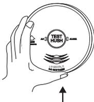
Slide Smoke Alarm cover in direction of arrow (as shown on cover) to remove from base plate
