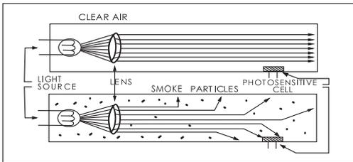
A light transmission source and a photosensitive receiver is used in this design. Light that is transmitted fall upon the receiver. When smoke or dust enters the light path, some of the light is scattered or absorbed. The result of a reduction of light falling upon the photosensitive receiver will cause an alarm.
